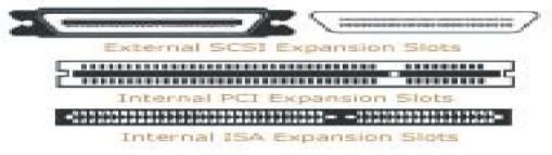
The previous pictures show the different types of slots on the motherboard for the component (card) to be added. When you want to install a card, you need only to look at the bottom of the card and match it to the same type of slot.
