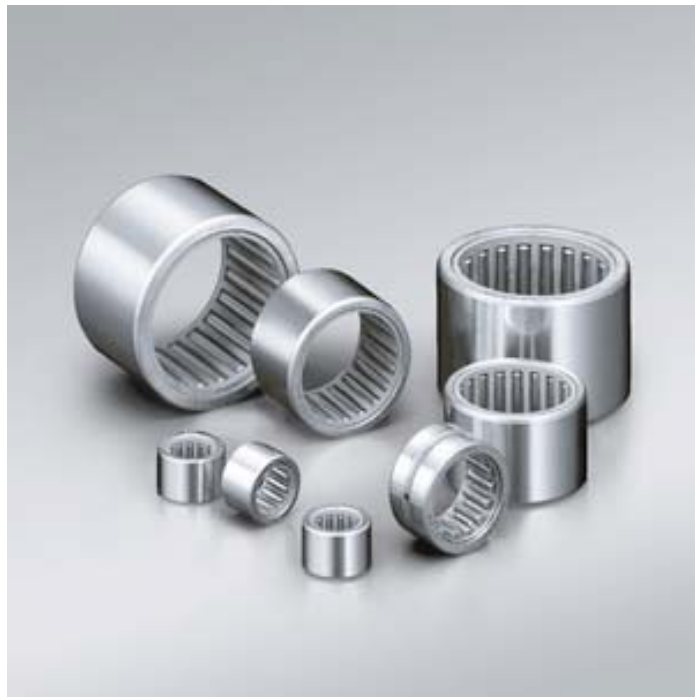
Figure 5-43 Examples of needle roller bearings. One of the main advantages of needle roller bearings is their small diameter, so they can be fitted into small spaces. They usually do not have a separate inner race, running directly onto the shaft, which must be suitably hard and with a precision ground surface. When these bearings fail, they often damage the shaft surface and the shaft needs to be replaced. Compare with ball and roller bearings, which have an inner race so that bearing damage is normally confined to the bearing races and the shaft is undamaged.
