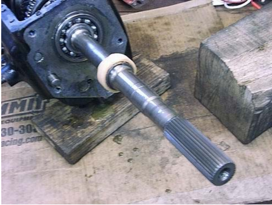
Figure 5-25 An example of a splined shaft from an automotive transmission (or gearbox). Details are not clear, but these splines are probably of INVOLUTE form (i.e. of the same shape as the involute gear teeth introduced in Part 4), since INVOLUTE SPLINES are easier to machine and are stronger than the square splines in Fig 5-24.
