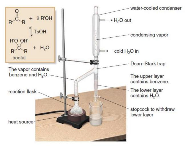
A Dean–Stark trap is an apparatus used for removing water from a reaction mixture. To use a Dean–Stark trap to convert a carbonyl compound to an acetal:
