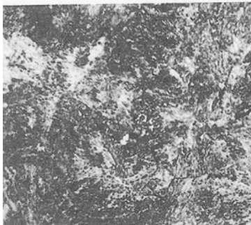
Figure 4-1 Carbon Steel Microstructures (These have been created in high carbon eutectoid steel [0.77% carbon] by isothermal transformation. A nital etchant and 500x magnification were used.) [11] Reprinted with permission of the American Welding Society. All rights reserved.
