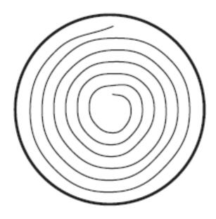
Figure 9: Spiral storage format for a CD.
